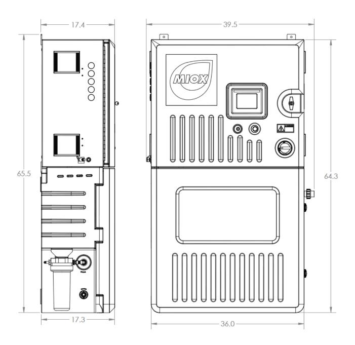
REFERENCE GENERAL ARRANGEMENT DRAWING 112-00001 FOR INSTALLATION REQUIREMENTS
